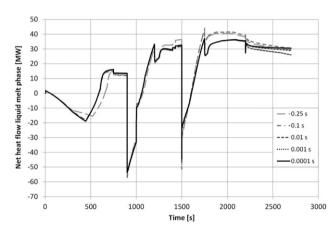
**Figure 5.** Net heat flow to liquid melt calculated with the Euler method.
