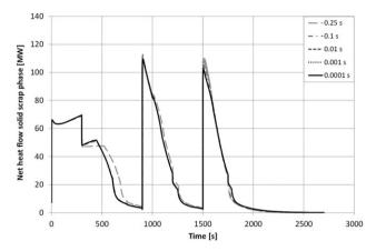
Figure 4. Net heat flow to solid scrap calculated with the Euler method.
