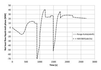
**Figure 7.** Net heat flow to liquid melt for Runge--Kutta(ode45) and NDF/BDF(ode15s).
