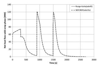
**Figure 6.** Net heat flow to solid scrap for Runge--Kutta(ode45) and NDF/BDF(ode15s).
